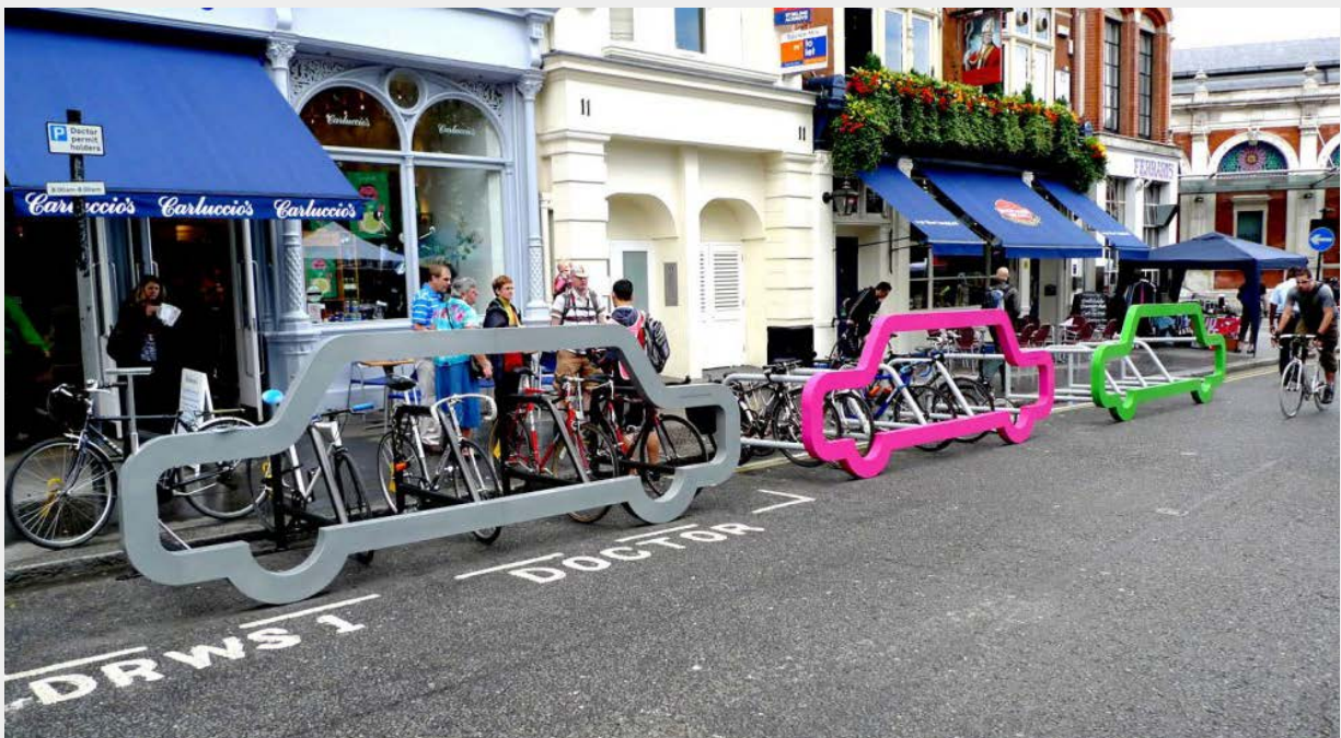
Figures 25, 26 and 27: Top two figures of Nagano train station in Japan which features significant bike parking infrastructure, making the last mile of the trip far easier. Bottom picture is of Cyclehoop bike parking which illustrates how many bikes can be docked in a single car parking spot.
